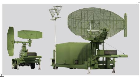
Is intended to ensure flight safety of aircraft and helicopters within terminal airspace, obtain positional information and guide aircraft to a safe landing in normal and adverse weather conditions. RSP-10MA consists of the surveillance radar (ASR) combining primary and secondary channels and Precision Approach Radar (PAR). Ground Controlled Approach System RSP-10MA is adopted by MoD of Ukraine for its Armed Forces.
