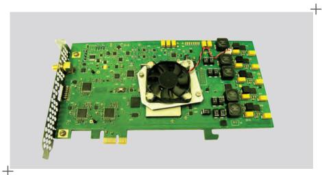
The demodulator was created and designed for functioning as a component part of a data receiving station from Earth Observation Satellites.
