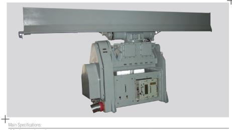
"Delta-M" is modern naval two-dimensional pulse coherent solid-state radar for surface and air surveillance with low probability of interception of its electromagnetic radiation.
